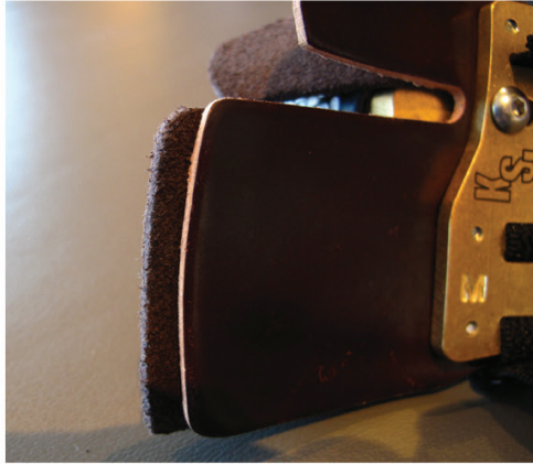
3. The trimmed edge on the backing needs to be one to two millimeters longer than the face.
