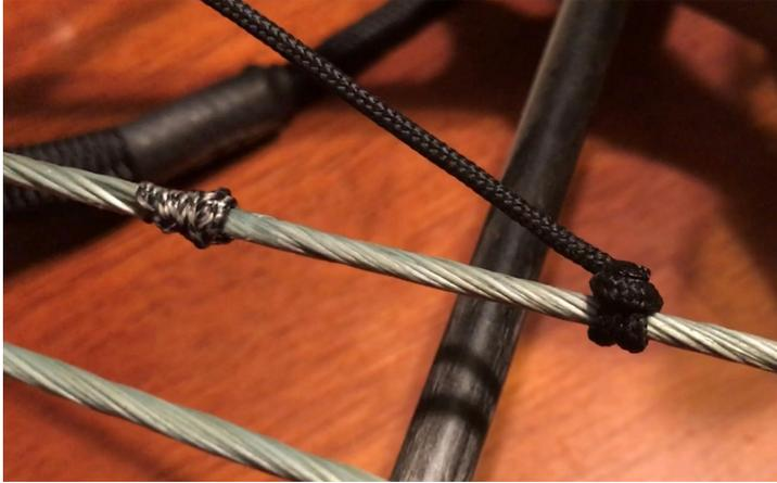
Slide the *activation cord* up to knot and adjust timing using *set screw* on the *activation knob* on rest. This installation method allows for easy in field servicing.
